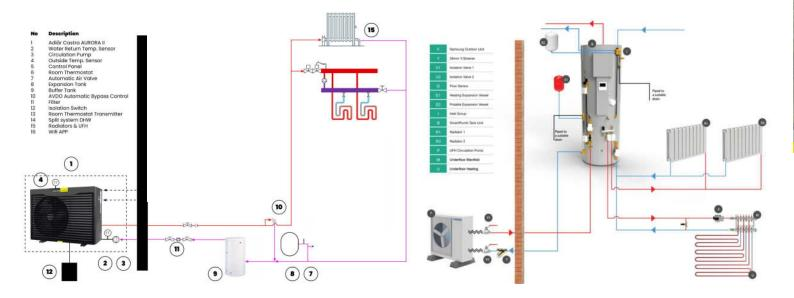
As you can see below, in the low loss header the return water also becomes warmer, which means (in this example) there is still only a 5°C temperature difference on the heat pump itself. However, as heat pumps work more efficiently at lower temperatures, heating 5°C to a lower temperature is more efficient than heating 5°C to a higher temperature.
